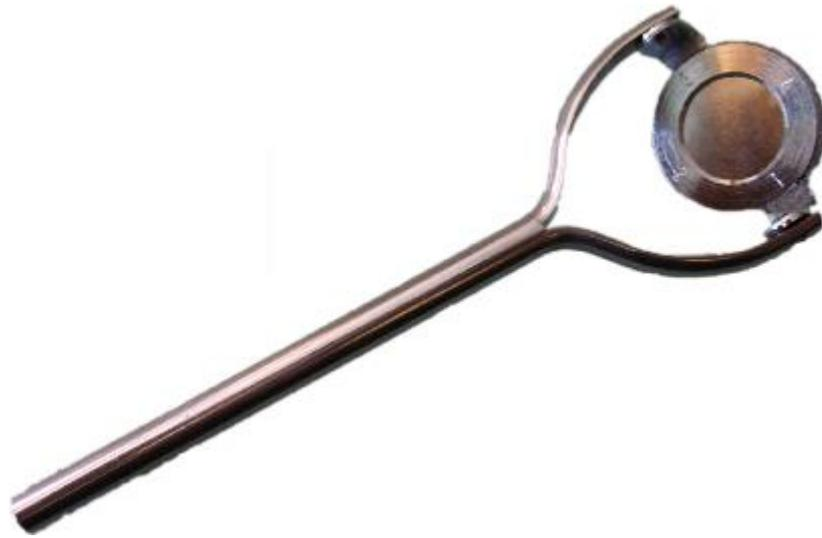
When placing on a magnetised test piece, magnetic lines pass through the sectioned iron cylinder. The cuts on the iron cylinder will be visible when magnetic powder or magnetic ink is applied. Maximum indication direction is achieved by rotating the penetrameter about its axis. The field direction is perpendicular to the flaw at maximum indication.
